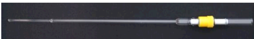
Figure 3.1.5.3 – Pressurisable stem co-axial insert for use with a standard 5 mm NMR tube.
