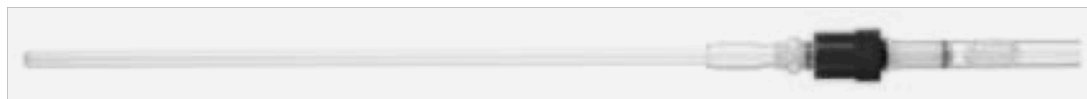
Figure 3.1.5.1 – A typical pressurisable NMR tube assembly with PTFE screw fitting allowing reduction / increasing of pressure to the tube inner. [137]
