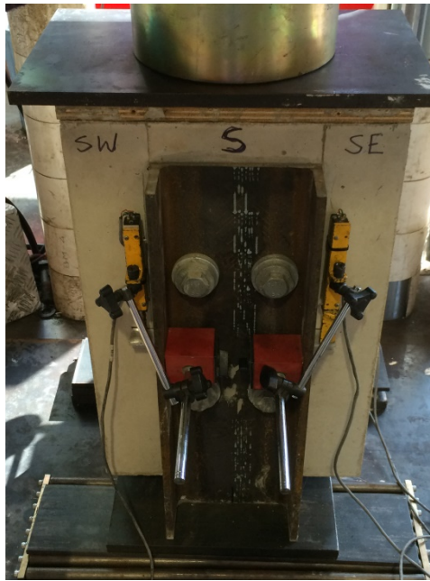
Figure 2. Push out test set up for ambient and post fire test specimens
