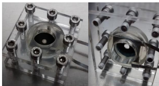
Figure 3-5. Photography of single chamber device, left: top view and right: bottom view.
