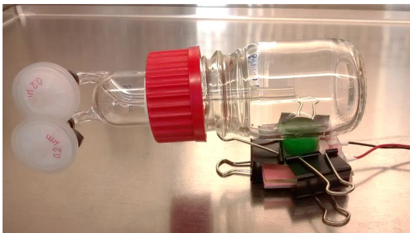
Figure 5-11. Photography of a nitrocellulose-MEA-BPV device for CO 2 enrichment inoculated with iron limited PCC7942.
