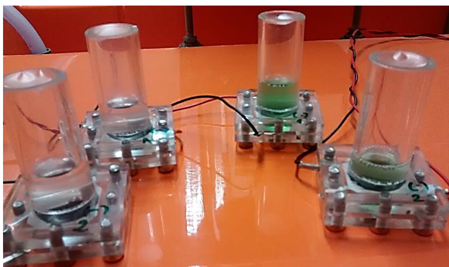
Figure 4-16. Photography of mediatorless MEA devices left for several weeks after characterised. Left: iron limited and Right: iron sufficient.
