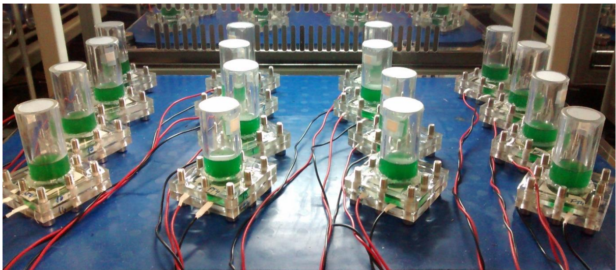
Figure 3-11. Photograph of nitrocellulose-MEA-BPV devices inoculated with PCC7942 (Day 1).
