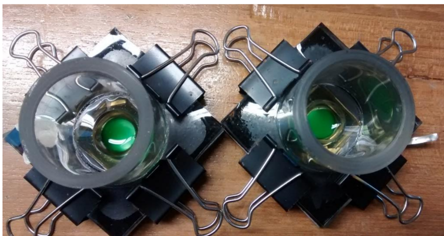
Figure 6-2. Photography of bioelectrochemical devices showing PCC7942 biofilms settled on the working electrode (ITO-coated glass) at the bottom of a 4 ml well.
