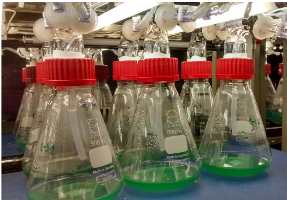
Figure 2-2. Photography of PCC7942 cultures grown under CO 2 enrichment, showing in and out connections.
