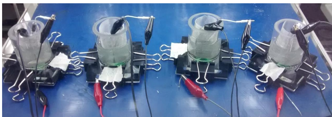
Figure 6-3. Photography of bioelectrochemical devices assembled with the biofilm on the working electrode, the reference electrode (Ag/AgCl) and the counter electrode (platinum mesh). Iron limited and iron sufficient biofilms under illumination incubated at 30 °C.
