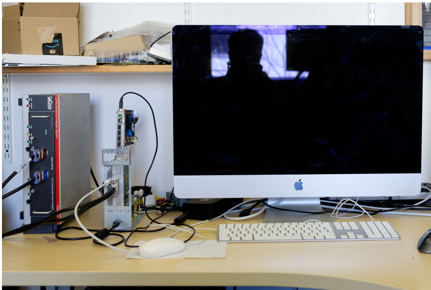
Figure 4.1: Photograph of macOS experimental setup. From left to right: the PCIe protocol analyser; the PCIe-Thunderbolt bridge, with the FPGA that runs the attack attached through a riser that connects to the analyser; the victim machine.
