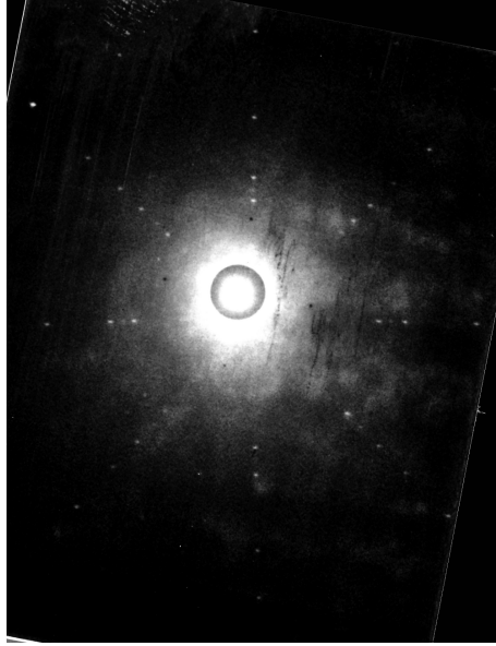
Figure 4.3: Single crystal Laue diffraction image obtained from the surface of a \text{YFe}_2\text{Ge}_2 piece.
