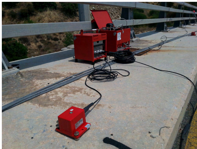
Figure 4.10: Uniaxial accelerometer, junction box, and unit including recorder, battery pack and GPS module
