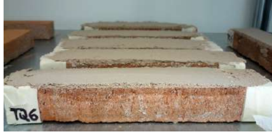
Figure 4: ARG TRM laminated brick specimens
