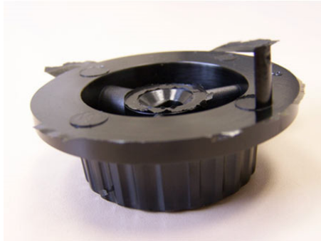
Figure 59 - Flash (Rebling Plastics)
