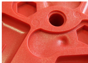
Figure 57 - Sink Marks (Rebling Plastics)
