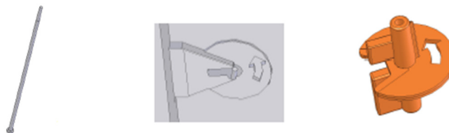
Figure 32 - (a) Core pin; (b) Core pin in mould cavity; (c) Moulded part (DS, Standard Components, 2008)
