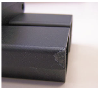
Figure 58 - Gas Marks (Rebling Plastics)
