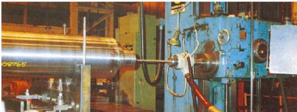
Figure 16 - A special machine tool with oil injection for horizontal deep hole drilling by ejector system. (DS, Deep Hole Drilling, 2008)
