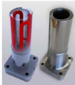
Figure 72 - Tool insert with conformal cooling channels
