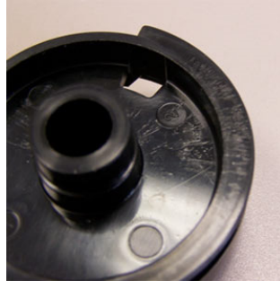
Figure 61 - Splay (Rebling Plastics)
