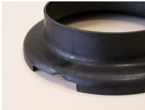
Figure 60 - Knit Lines and Short Shot (Rebling Plastics)
