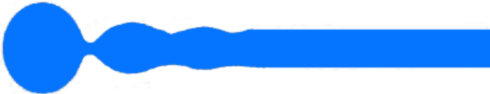
Fig. 2.5: Schematic illustration of the rim shape regime obtained for a retracting sheet (side view) at Oh < 0.1 . Adapted from Brenner & Gueyffier [25].
