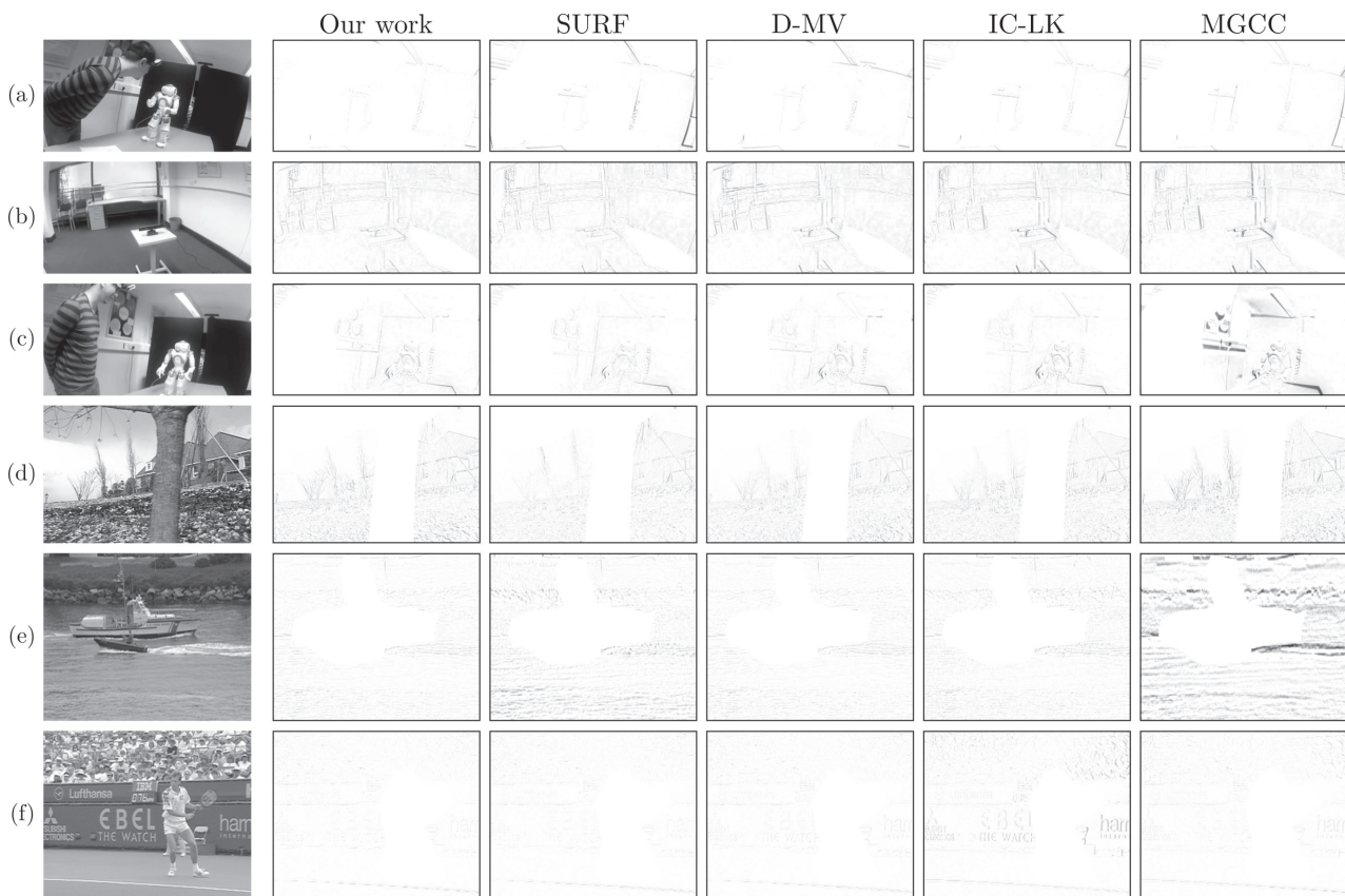
Fig. 8. Exemplar frames from test sequences and the corresponding difference images obtained after global motion was compensated with each of the methods. To enhance the interpretation of the difference images, we segmented out the largest moving foreground object from difference images manually and also inverted the difference images in color. (a) Ego-centric1, the SURF method in this frame was affected by barrel distortions which caused higher noise near the edges of the difference; (b) Ego-centric2, a scene with a large number of lines curved by barrel distortion; (c) Ego-centric3, a scene with barrel distortions and large outlier motions; (d) Flower, a scene with elements of varying depth; (e) Coastguard, two (visually salient) ships are moving towards each other; (f) Stefan, a sequence where the tennis player causes large outlier motions.
