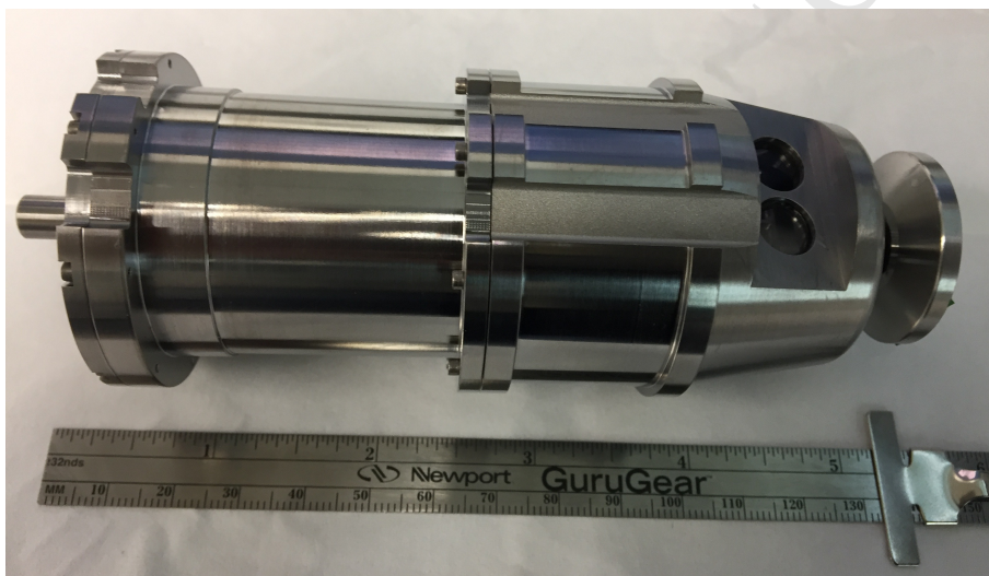
Figure 9: Saturn probe prototype NFR vacuum micro-vessel with sapphire and diamond windows; this houses a focal plane assembly that accommodates Winston cones with a 5^\circ field-of-view acceptance angle.
