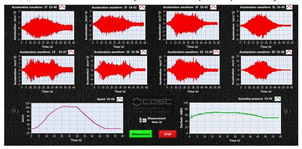
Figure 6 Example of the data gathered in LabView environment during an operational test between 0-60 s: the 8 acceleration signals are displayed at the top; the speed of the car is displayed at the bottom left; and the sound pressure level in dB(A) at the driver's ear is provided at bottom right.
