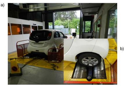
Figure 5 Photographs of the electric vehicle mounted on the chassis dynamometer (roller bench): a) vehicle in the laboratory; and b) the rear wheel on the rollers.
