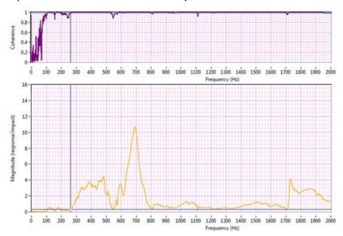
Figure 4 Static FRF impact tests: an example of the measured FRF with the accelerance amplitude at the bottom and the corresponding coherence at the top.
