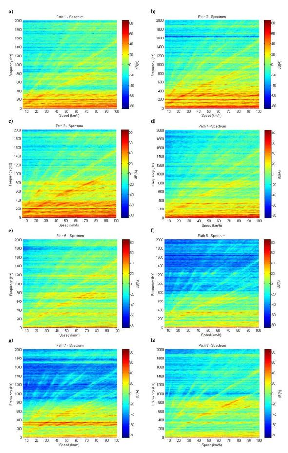
Figure 18 STFT showing the sound pressure level in dB(A) due to each transfer path against frequency and vehicle speed calculated using TPA: a)  $1^{st}$  path; b)  $2^{nd}$  path; c)  $3^{rd}$  path; d)  $4^{th}$  path; e)  $5^{th}$  path; f)  $6^{th}$  path; g)  $7^{th}$  path; and h)  $8^{th}$  path.
