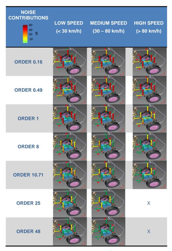
Figure 22 Contribution of each path (1 to 8) calculated using the TPA and agreement ( $\checkmark$ ) and discrepancies (\*) with the corresponding OPA result at the dominant engine orders in the low, medium and high frequency ranges.
