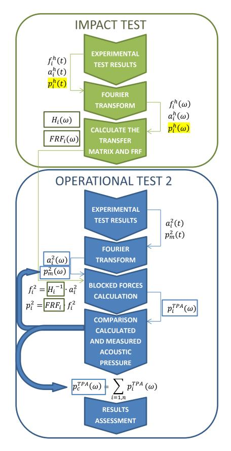
Figure 16 Flowchart illustrating the procedure for Transfer Path Analysis (TPA).
