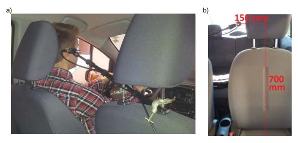
Figure 3 The microphone location near the driver's ear: a) vehicle interior; and b) location relative to driver's seat.
