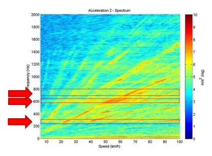
Figure 7 Short Time Fourier Transform (STFT) for the signal from accelerometer 2Y.
