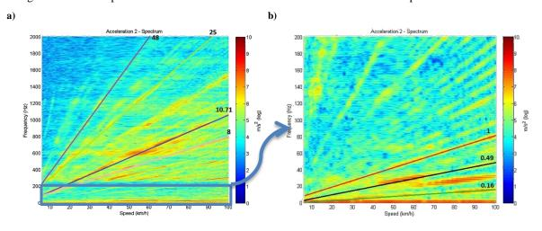
Figure 8 STFT illustrations of the engine orders for the signal from accelerometer 2Y: a) 0 to 2000 Hz; and b) 0 to 200 Hz.
