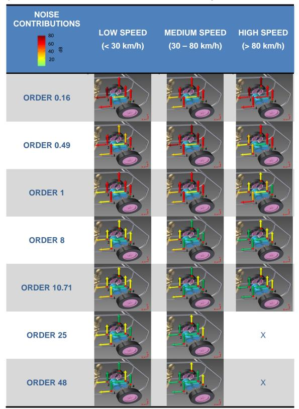
Figure 15 Summary illustrations of the relative strength of each path (1 to 8) calculated using OPA at the dominant engine orders in the low, medium and high speed ranges.
