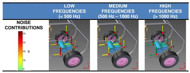
Figure 19 Summary Illustrations of the contribution of each path in the low, medium and high frequency ranges calculated using TPA.
