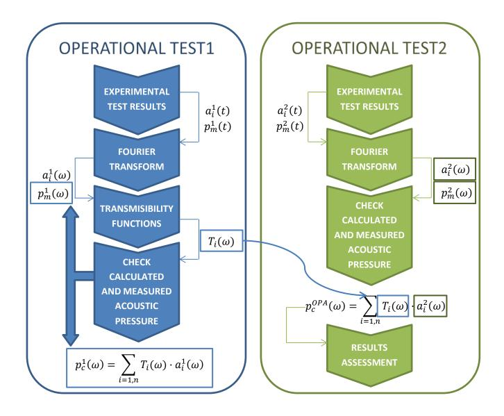
Figure 9 Flow diagrams illustrating the procedure for Operational Path Analysis (OPA).
