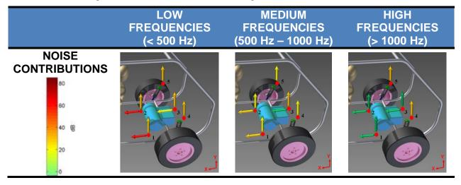
Figure 13 Summary illustrations of the relative strength of each path in the low, medium and high frequency ranges, as calculated using OPA.
