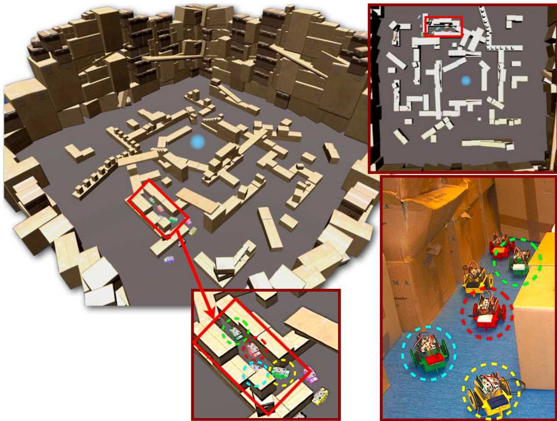
Figure 4: Computational and real-world experiment about the problem of finding a target location for swarm robotics: general view (top-left), top view (top-right) and selected regions of interest (bottom-middle & right).
