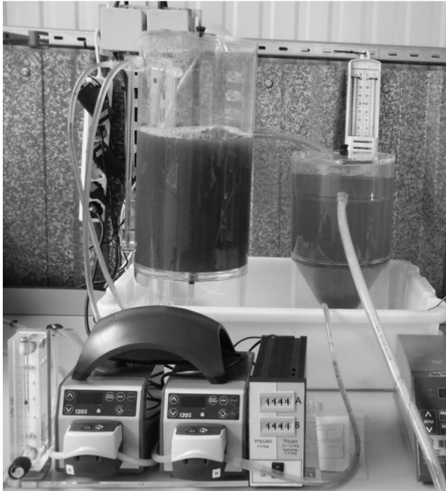
Fig. 1. Equipment of biological treatment with activated sludge.
