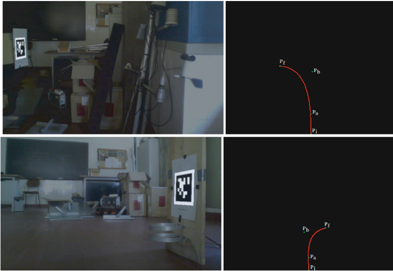
Fig. 4. Detected tag (left) and Bezier Curve obtained (right).
