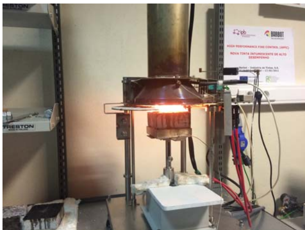
Fig. 5 – Ignition of epoxy resin from an unprotected specimen
