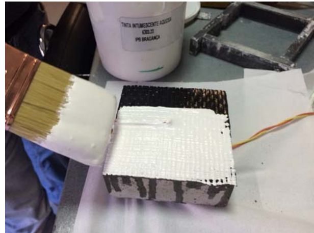
Fig. 4 – Application of the intumescent paint
