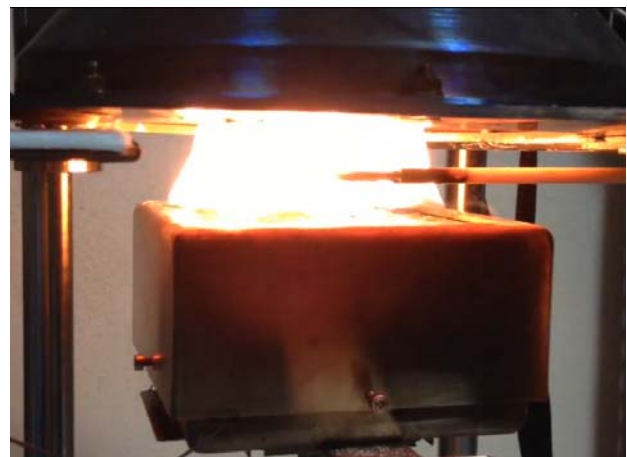
Fig. 10 – Ignition of intumescent coating
