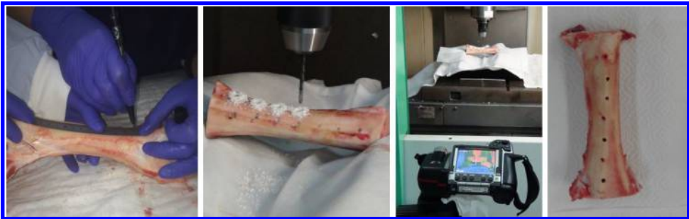
Fig. 3. Drilling operations of bovine bones.
