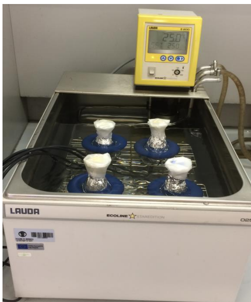
Figure 3.1: Experimental setup of the shake-flask methodology.
