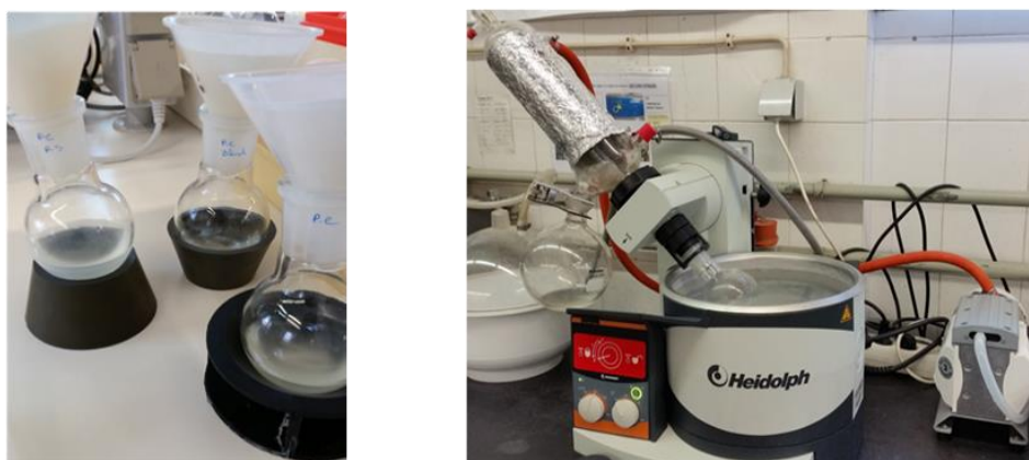
Figure 11. Step of solvent removal in the preparation of the extracts.
