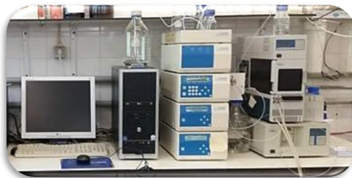
Figure 12. HPLC system used in tocopherols analysis.
