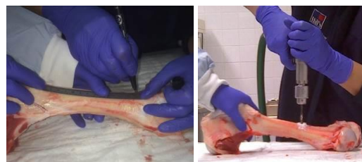
Fig. 3-Marking of the holes and drilling process.
