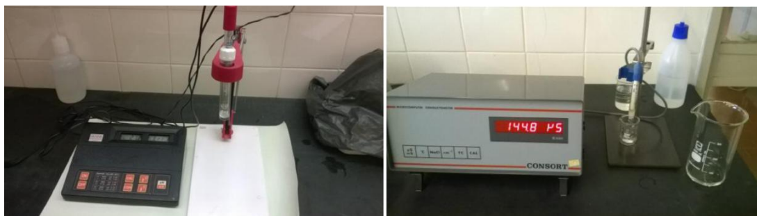
Figure 3.5. Instruments used for water parameters measurements: (a) pH (HANNA instruments HI8417); (b) conductometer (Consort K320)
