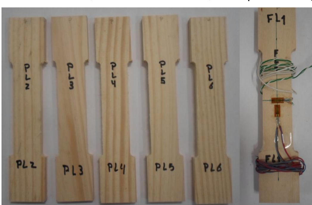
Figure 3 - Test samples and strain gauges instrumentation.
