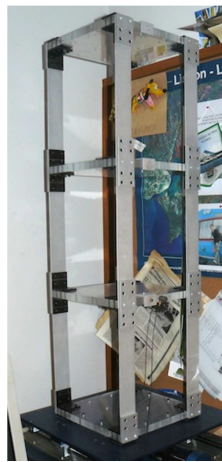
Figure 2: Metallic scaled frame at the shaking table.
