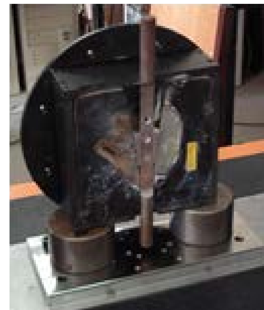
Fig. 1. Apparatus used for measuring deformations on the bone-implant interface.
