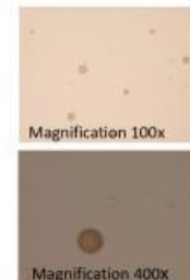
Figure 6. PUD nano-in-micro particles obtained by atomization in a Var J30 microencapsulation unit.
