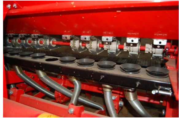
FIGURE 4: Seedbox bottom and seed tubes
