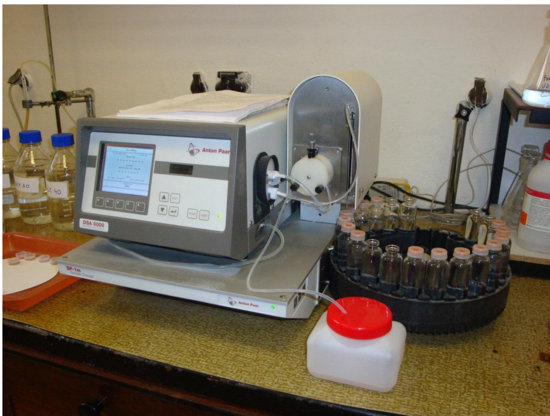
Figure 3.1. Experimental apparatus: density and sound velocity meter DSA 5000 from Anton Paar.
