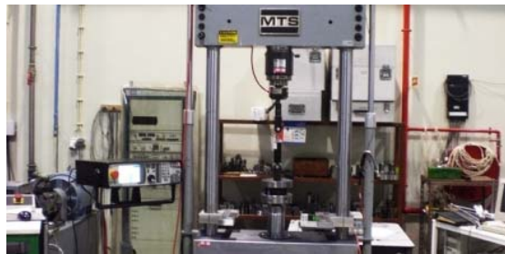
Figure 39: Magneto-rheological damper with current supply device, connected to MTS universal setup (FEUP).
