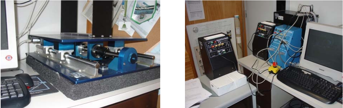
Figure 43: Quanser shaking table II (and its controllers) at FEUP – Covicocepad Lab.
