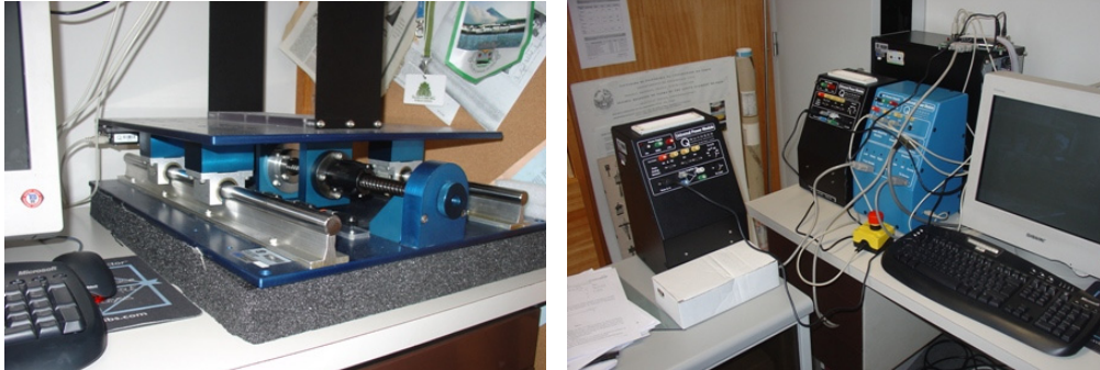
Figure 12: Quanser shaking table II (and its controllers) at FEUP – Covicoepad Lab.
