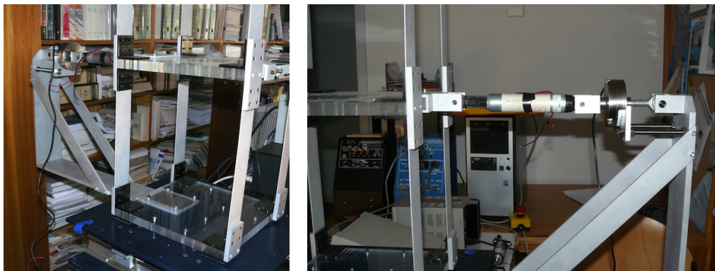
Figure 13: MR damper attached to the experimental metallic frame.
