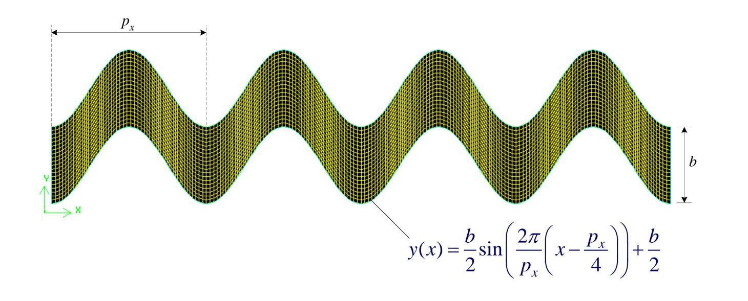
Plate width >>  $b \Rightarrow 2D$  channels
