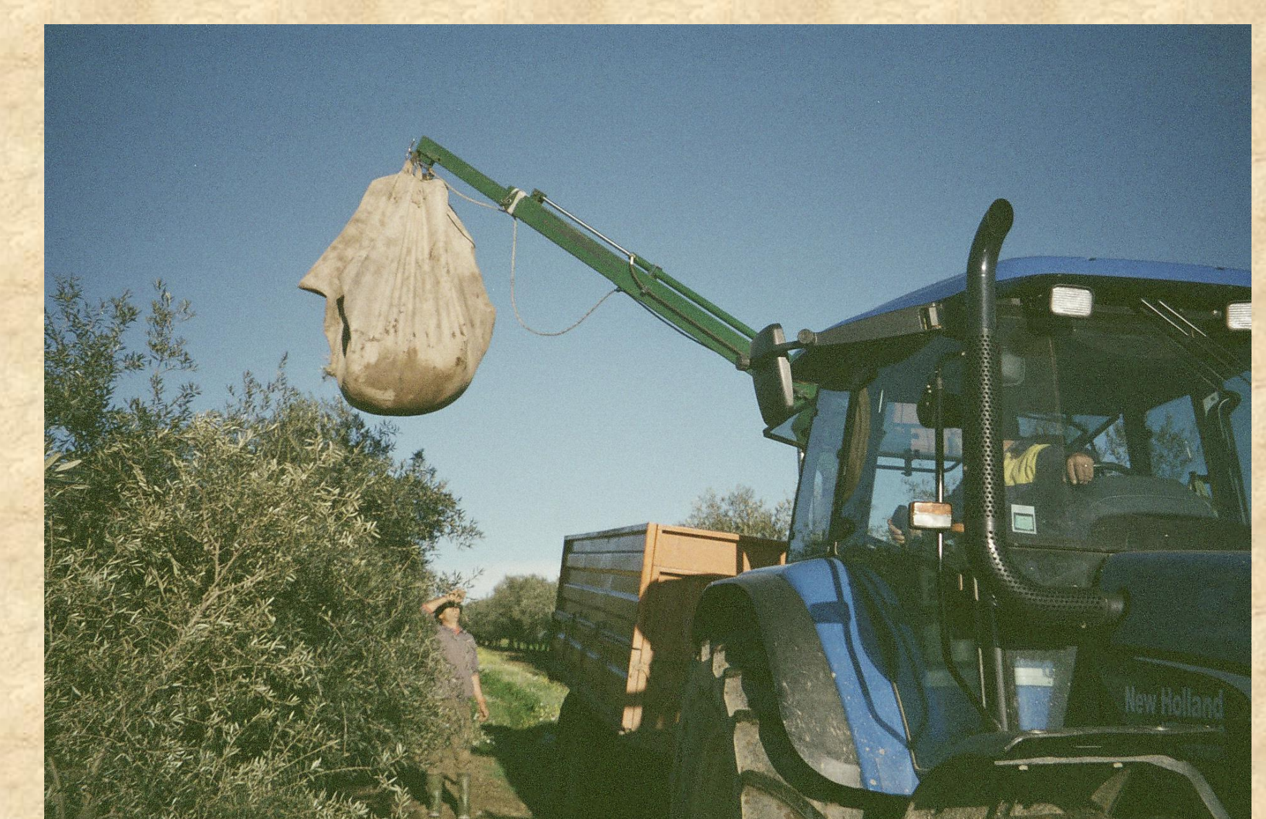
Fig.7. Rear mounted hydraulic crane, loading olives.
