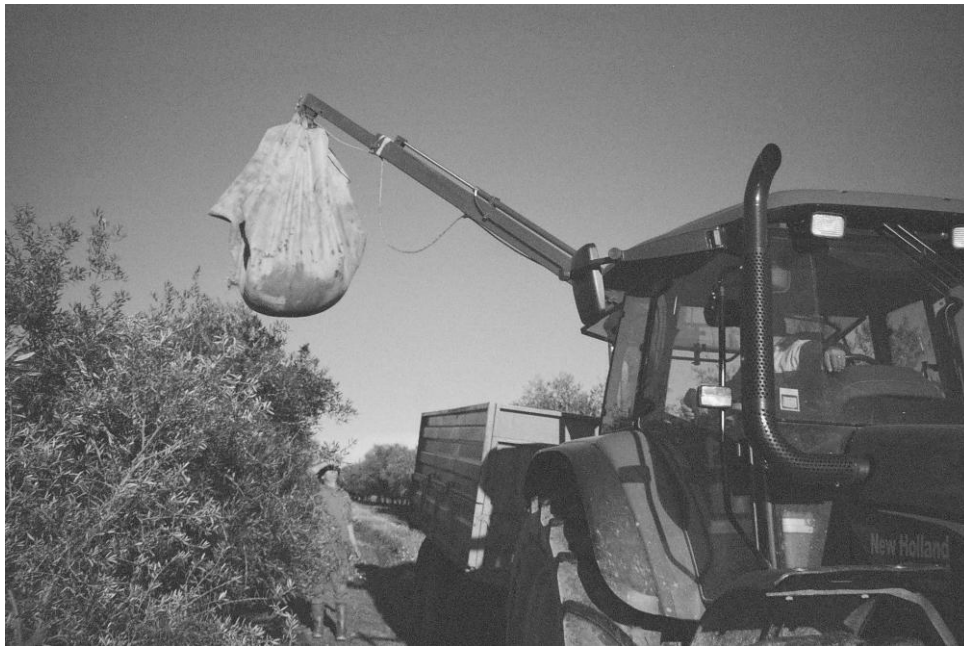
Fig.4. Rear mounted hydraulic crane, loading olives.
