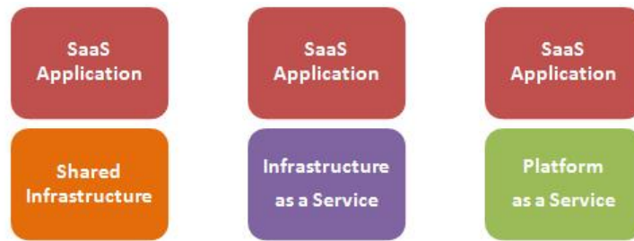
Figure 2.4: Three ways to host a SaaS Application [Keith, 2009]
