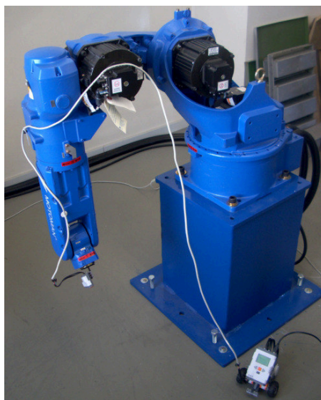
Fig. 15. Industrial robot placing the ultrasonic sensor.
