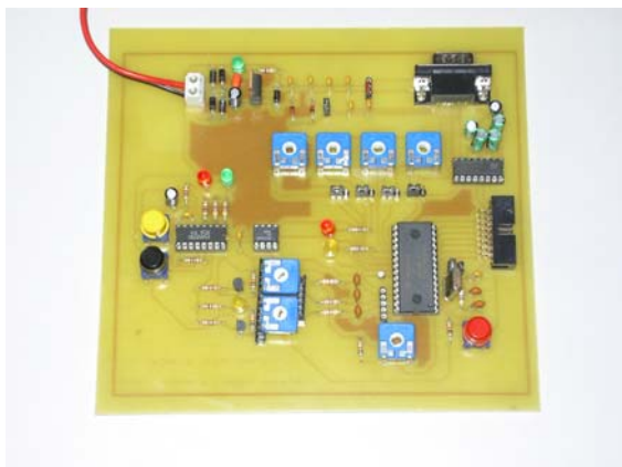
Figure 3: The controller board based on MC3PHAC.
