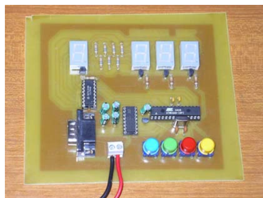
Figure 4: The master board using the Atmega8.
