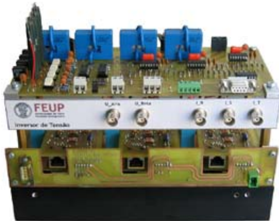
Figure 5: Voltage source inverter and measurement board implemented as described in [8].
