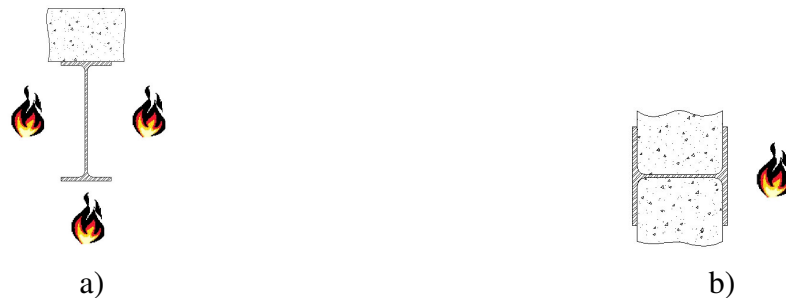
Fig. 6 – a) Beam subjected to fire in three sides; b) Column subjected to fire in one side.
