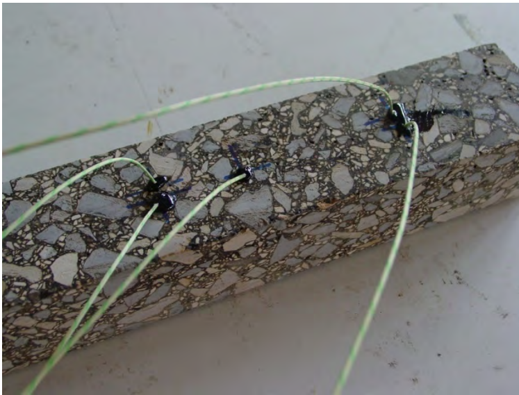
Figure 14. Test sample with thermocouples for temperature measurement
