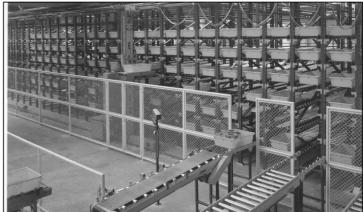
Figure 2.8: Automatic Storage and Retrieval Systems
