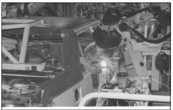
Figure 2.6: Industrial Robot in Materials Handling and Welding Tasks
