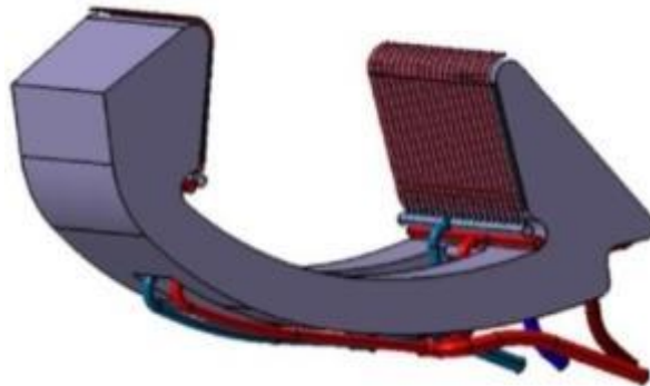
Figure 55. First cooling configuration option. The colour of the pipes depends on their role: the blue for inlet pipes, red for the outlet ones.
