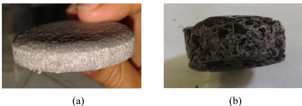
Figure 3.15 Geopolymeric foam samples produced using SS solution with R=3 (a) and R=2 (b)
