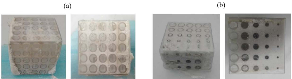
Figure 5.44 Templates impregnated with D-HCF/100 foam after curing
