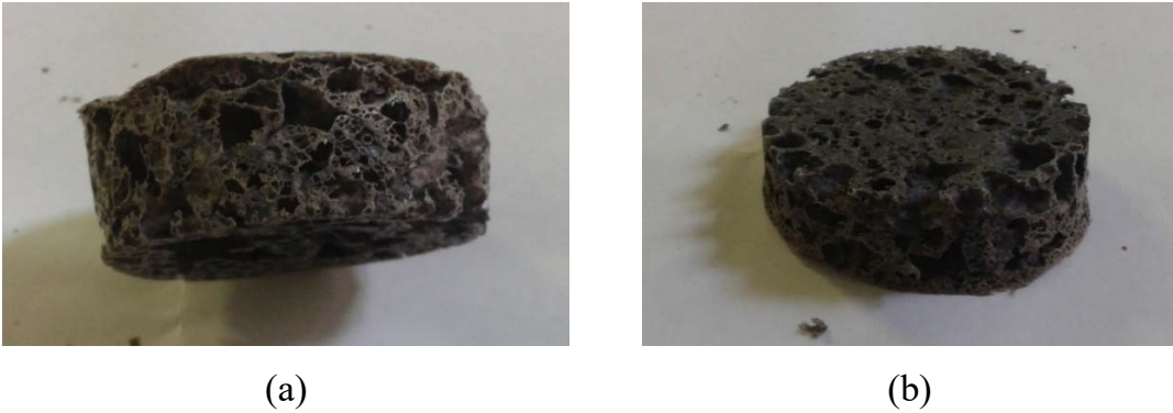
Figure 3.17 Geopolymeric foams cured at the temperature of 40°C (a) and of 70°C (b)
