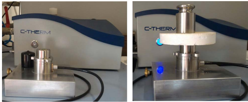
Figure 5.28 Thermal conductivity analyzer used for thermal conductivity measurements
