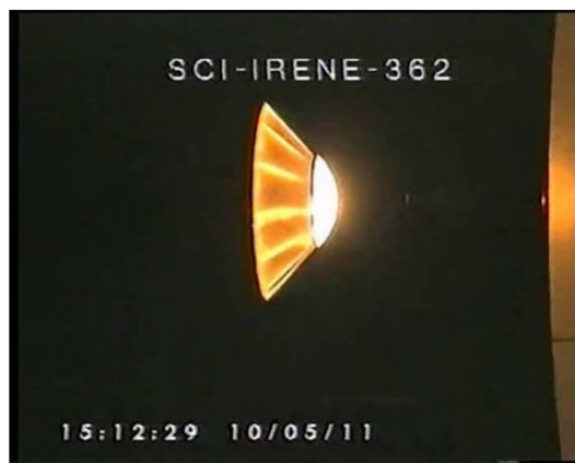
Figure 2.2.7 - Test article at the end of the PWT test [22].
