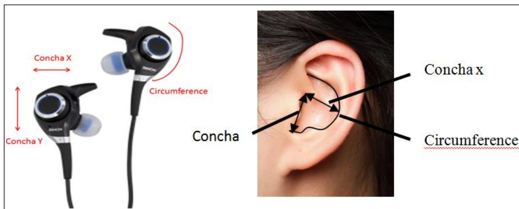
Figure 2. An image of the prototype and respective critical ear dimensions
