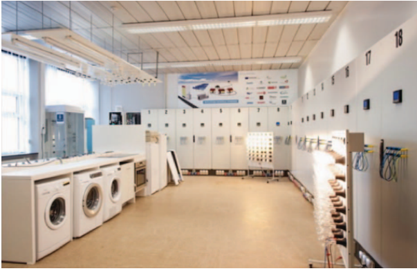
Fig. 3. The experimental grid laboratory. Each of the 18 numbered cabinets represents a domestic consumer.
