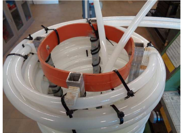
Figure 1 Picture of the studied helical coil heat exchanger.
