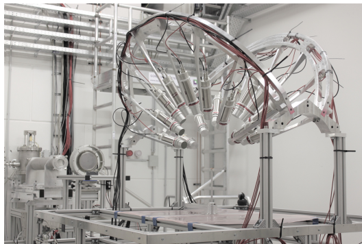
(b) Picture of the setup installed in the nELBE measurement hall for the iron measurement. Here the beam comes from the left. In front of the beam exit the PTB fission chamber is seen. The JRC fission chamber is upstream, just behind it.
