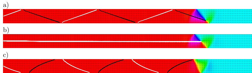
Figure 11. The path of a vortex core in a permalloy nanostrip where the vortex domain wall is driven above the Walker breakdown/depinning current threshold by a spin-polarized current with (a) \beta = 0 , (b) \beta = \alpha and (c) \beta = 2\alpha .
