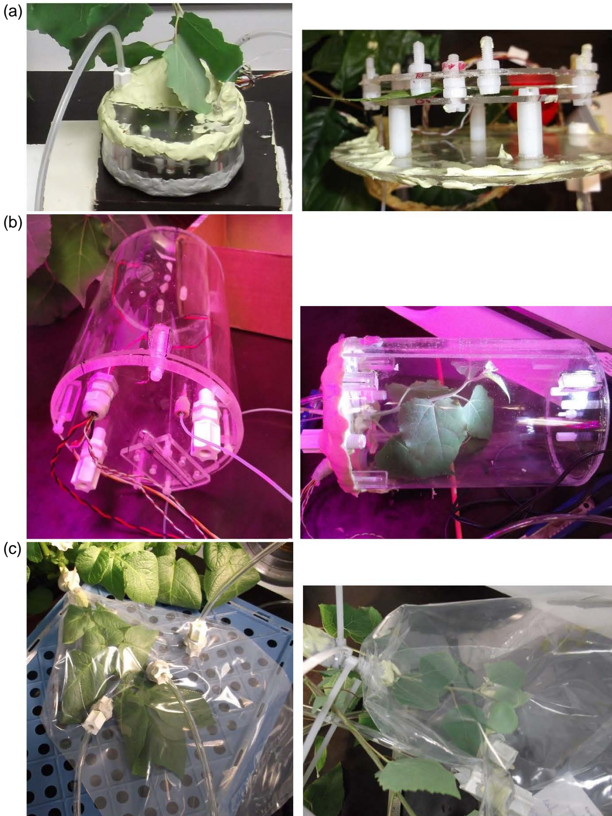
Figure 5.2 Different cuvette designs to administer gaseous ^{11}\text{CO}_2 to leaves attached to intact branches. (a) Small plexiglas cuvette in which one or two leaves could be fixed between two plexiglas plates, serving as positron shields (Text box 4.1). (b) Larger plexiglas cuvette without positron shields that could fit an entire distal part of a branch with multiple leaves. (c) Versatile and airtight branch bag (details in Chapter 6).
