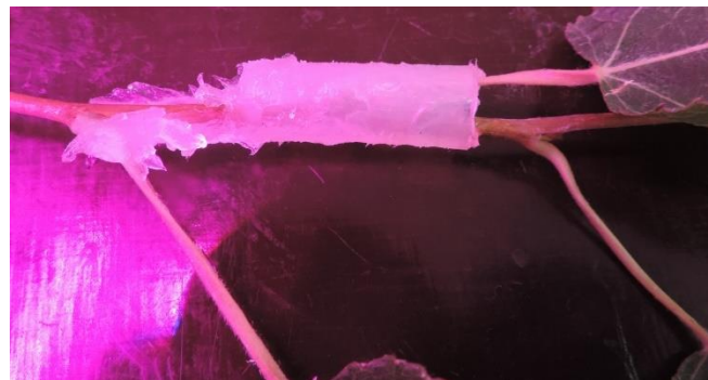
Figure 6.3 Detail of the plastic tubing, covered with vacuum grease on the inside and encapsulating the intact branch to ensure an airtight seal without damaging the branch surface.
