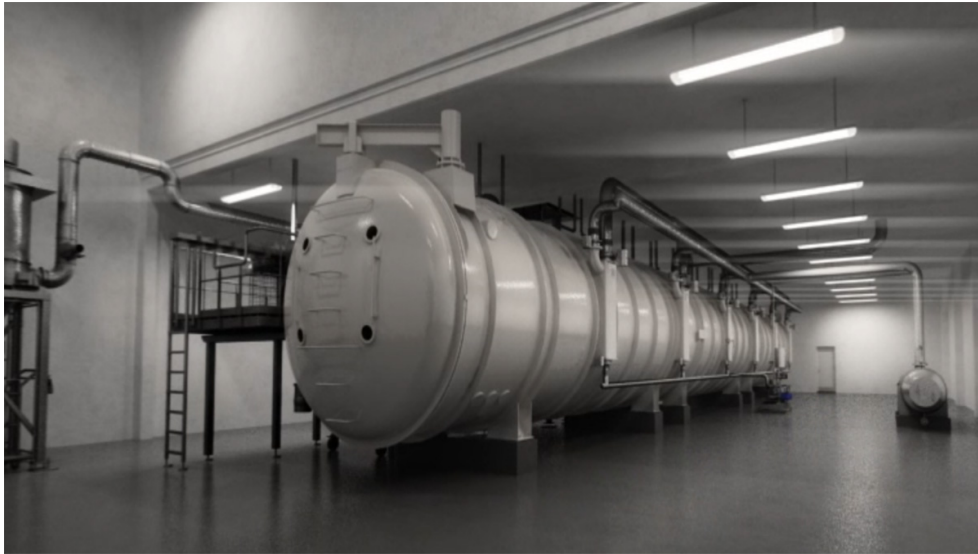
Figure 5.1: The CONRAD™ freeze-drying plant from GEA Group [11]
