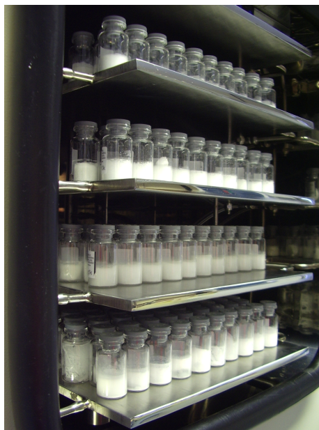
Figure 1.1: Temperature-controlled shelves loaded with vials in the drying chamber of a pilot-scale batch freeze-dryer
