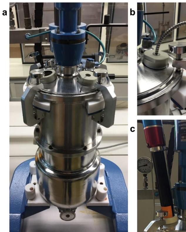
Figure 1. Experimental setup: (a) customized mixing system without probes; (b) UV immersion probe; (c) Raman PhAT probe.
