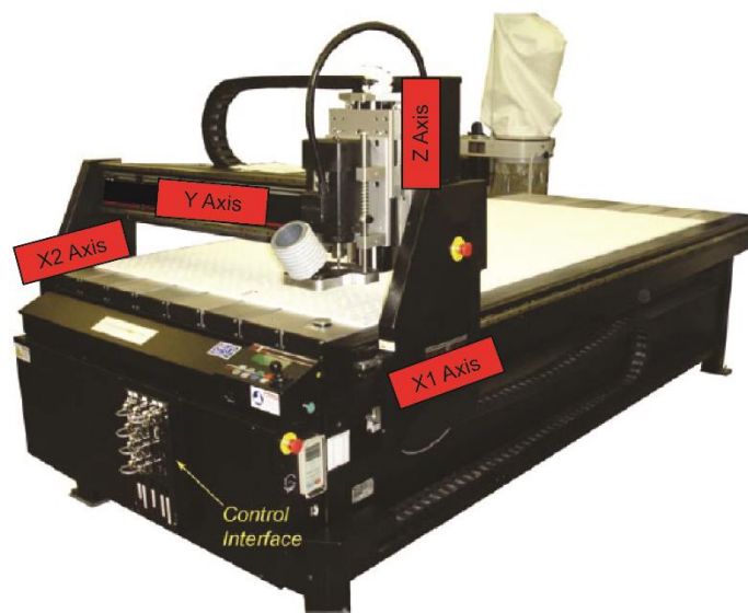
Figure 6-1 Experimental setup (4'x8' wood router table)
